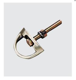
**D-Bolt Anchor**For up to 4 inches (102mm) working thickness. Includes a 0.63 inch (16mm) diameter bolt with lockwasher and nut.
